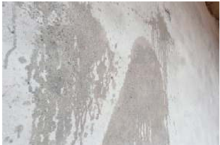
Plaster with RenderCon '5S' demonstrating hydrophobicity
